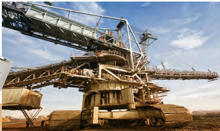
*Bucket wheel excavator with conveyor belt*
